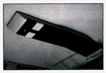
The optional roof console has two storage compartments. To open the compartments, push up and slide the door forward. To close the compartments, slide the door back. Use the straps to secure items.
